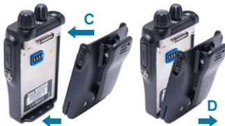
1. To attach (C), locate the pegs on the bottom of the battery into the slots on the radio and pull the 2 latches downwards, carefully pushing the battery into the radio. Ensure the battery is full attached.
