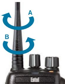
1. To attach, carefully align the antenna with the socket. Screw in the antenna and clockwise (taking care not to cross the thread) until it is seated firmly. (A)
