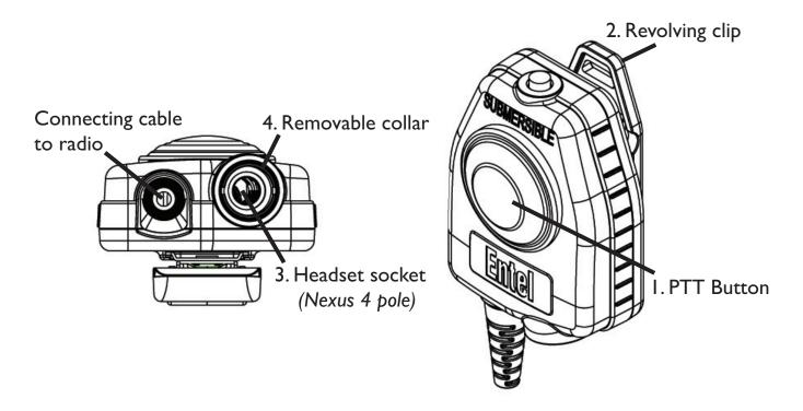
Always switch the radio off before attaching an audio accessory and fit only outside of I.S area
