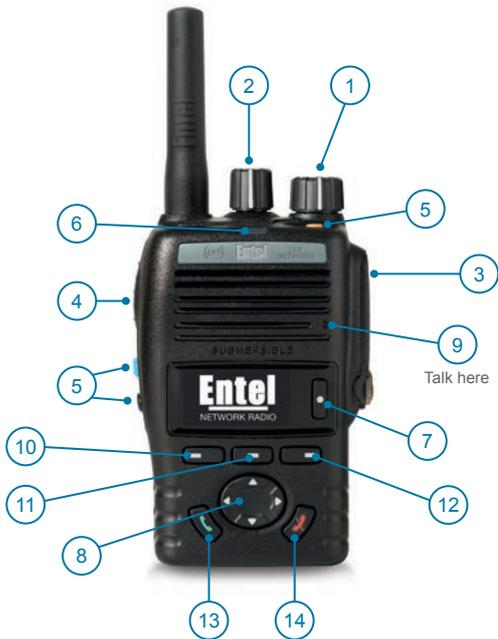
1. On/Off/Volume control. Rotate clockwise to turn on and increase volume. Rotate anti-clockwise to reduce volume & turn off.
