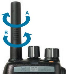
1. To attach, carefully align the antenna with the socket. Screw in the antenna clockwise (taking care not to cross the thread) until it is seated firmly (A).
